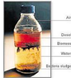
A sample of red diesel showing the formation of bacteria sludge.
